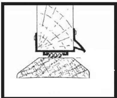
Illustration shows two ways to use hardwood threshold. Measure door opening between jambs and cut to fit with saw. For neatest job, cut threshold to fit around door stop. Or cut door stop to fit threshold.
