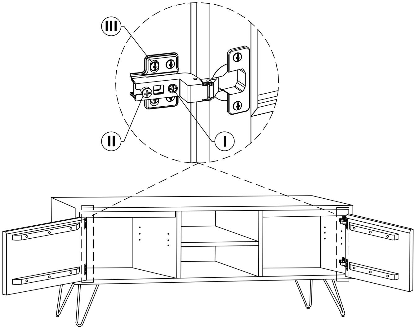
Tighten the Screw marked ② to fasten hinge. The door may need to be adjusted so that all the spaces between the door and the unit sides are equal. to adjust, follow instructions:
