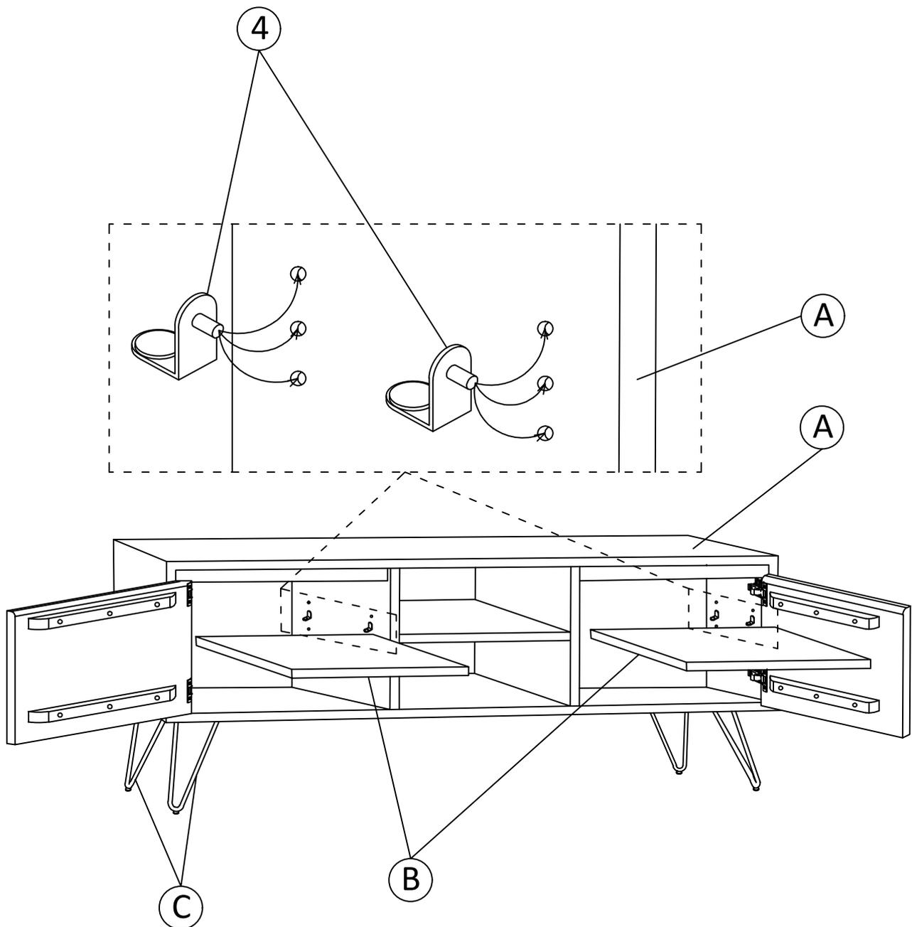
1. Insert four shelf supports ④ into the holes of both cabinets of top ①.
