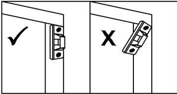
2. Determine where furniture is to be placed and mark location on the wall for mounting bracket screw hole approximately 2 inches **below** the bracket mounted to the furniture.
