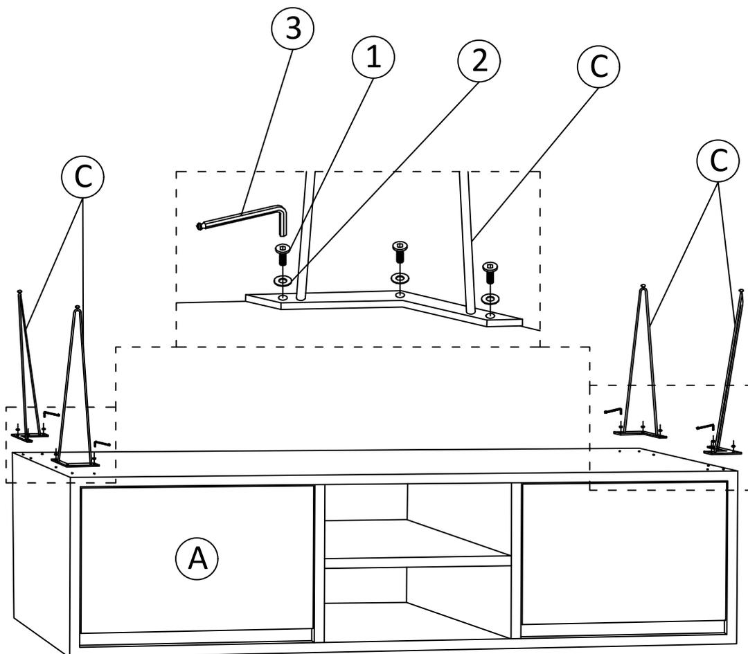
1. Attach Legs (C) to Top (A) with Allen key Bolts (1) and Washers (2) .
