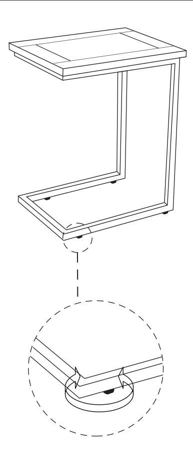
Note: Levelers underneath the base can be adjusted if floor is uneven.
