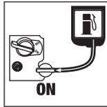
**9****Verify the Engine Switch is turned to the ON Position**
