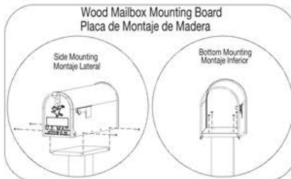
To install onto a wood mounting board use a #8 x 1-1/2" wood screw. To install onto a Gibraltar Mounting Bracket (sold separately) see above.
