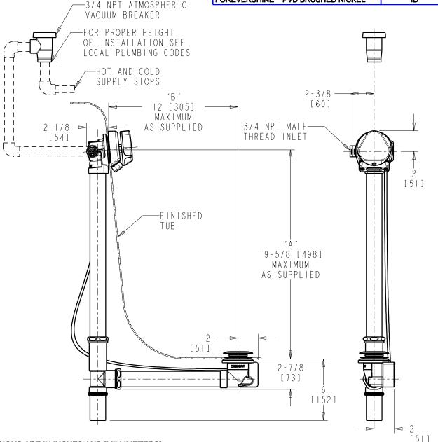
DIMENSIONS ARE IN INCHES AND [MILLIMETERS].
