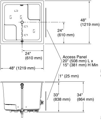
No change in measurements if connected with drain illustrated. (K-8150)
