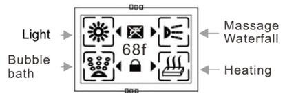
For the model with heating function, the temperature flickering is preset temperature; the one showed constant is actual temperature.
