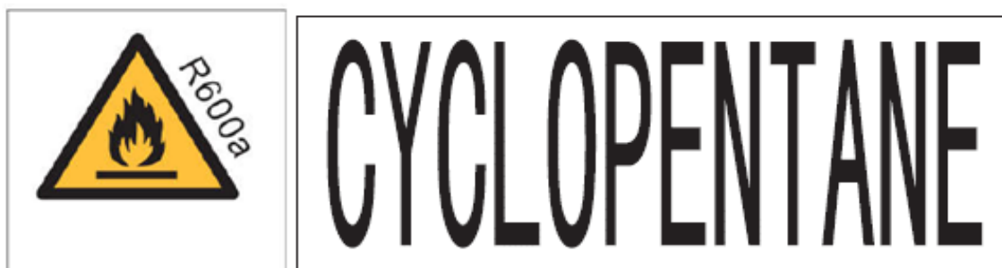
Illustration 1.2 - Marking for flammable insulation blowing gas type
