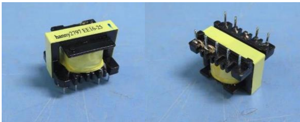
Photo 59 - View of transformer model EE16-25
