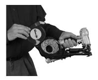
Place cap reel in basket. Make sure the front end of the cap coil is placed over the cap guide area of the basket. Insert lead cap into the feed chute.
