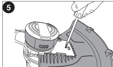
The locking tab (10) should be snapped into the housing slot (11).
