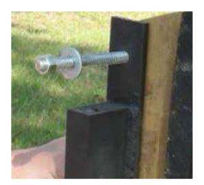
The frame bracket with the longer middle bar is on the hinge side during installation. The plates should be closest to the outside of the gate.
