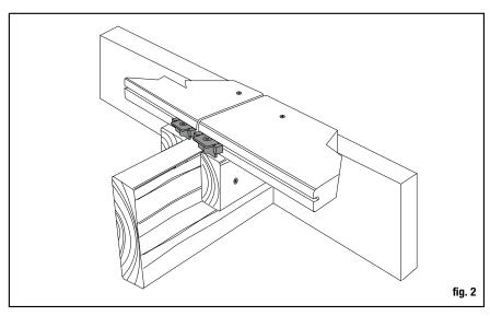
Fasten the outside edge of the first board to the rim joist with screws. Pre-drill and countersink all deck screws, regardless of type, that are within 1-1/2" of the end of the deck board. On the other side of the board, place a Stowaway hidden fastener into the slot and center on the joist.
