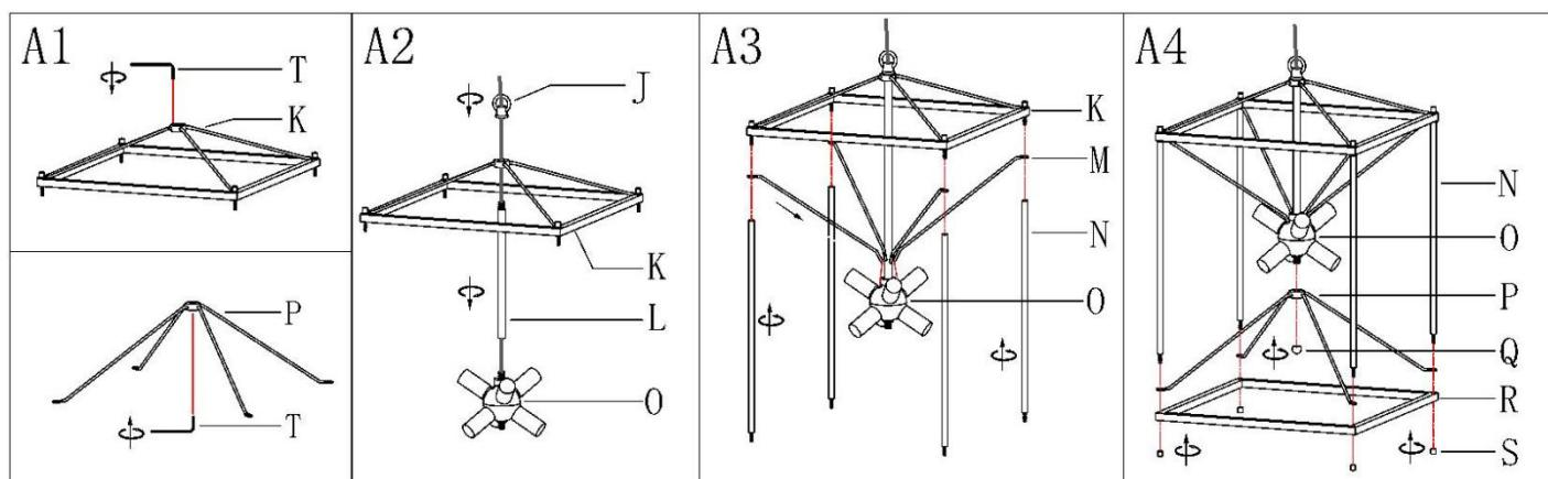
**Step A1 »** • Check that the arms of upper frame (K) and iron rack (P) should be secured.
