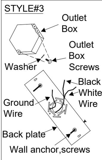
Style#3: Remove screws from outlet box. Attach full size back plate by putting the outlet box screws on screws included through the back plate and tighten.
