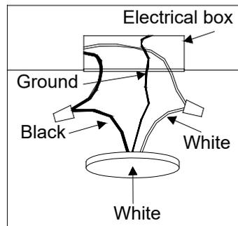
4: Feed the black or red wires, white wires and ground wire through the hole on the backplate. Then proceed by connecting black wire or red wire from outlet box to black wire on fixture, connect white wire from electrical box to white wire on fixture. Connect ground wire from outlet box to the ground wire on fixture.
