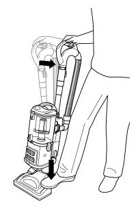
**3** Gently step on the floor nozzle and tilt the handle back.
