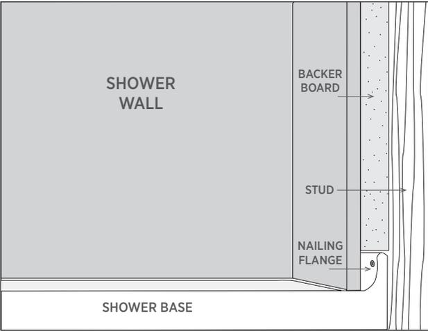
The diagram shows a cross-section of a shower wall assembly. From left to right, it labels the SHOWER WALL, BACKER BOARD, STUD, and NAILING FLANGE. Below the wall assembly is the SHOWER BASE. The nailing flange of the shower base is shown attached to the stud, with the backer board extending down to rest on the base.
