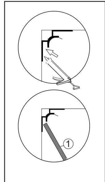
6. Press against the wall smoothing out any air bubbles along the entire area and then lightly tap on wall panel with a rubber mallet from top to bottom to ensure it is tightly connected to the wall.
