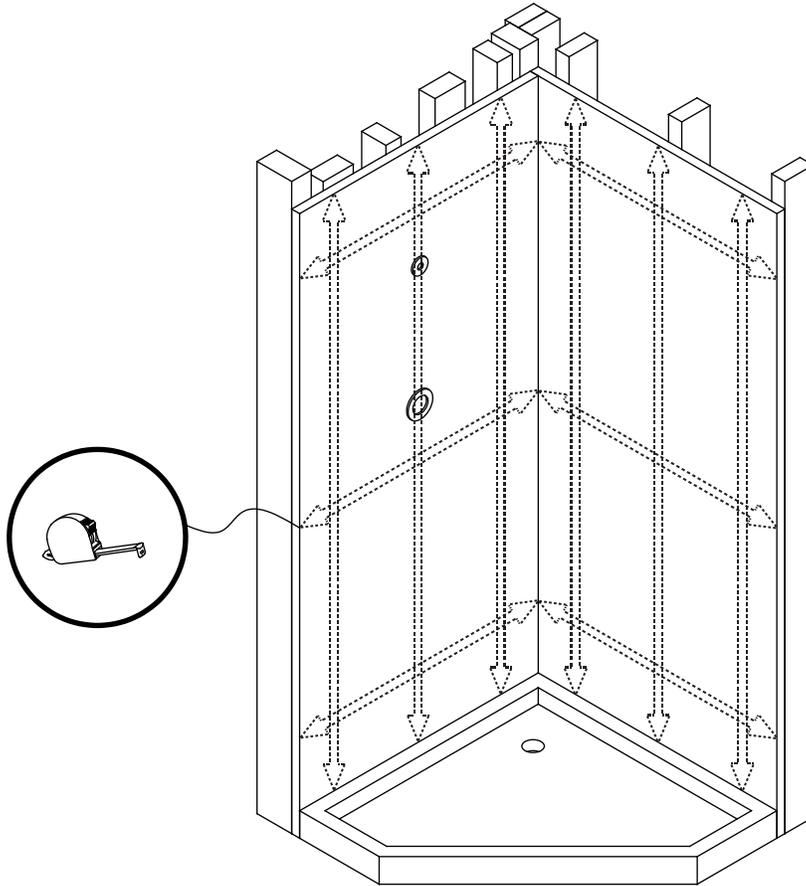
3. Measure cut-out locations for plumbing fixtures and mark them on the back of the appropriate panel(s).
