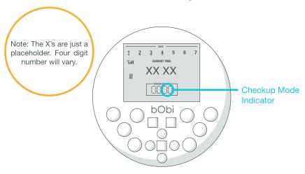
Press RGHT on bObi's remote to cycle through each step of the checkup test. Press LEFT to alternate between subsections of each step. The checkup mode indicator shows which step of the test bObi is in.
