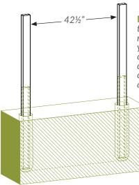
Note: If you intend to remove and reinstall the gate, you can substitute concrete with crushed stone compacted tightly around the posts.
