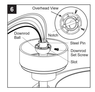
Insert downrod ball from downrod pack (E) into the opening of the mounting bracket (A). Rotate the downrod ball until the tab in the mounting bracket (A) is seated in the slot in the downrod ball.
