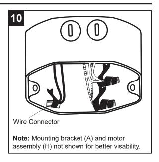
Connect the pin connectors on the wires from motor assembly (H) to the connector ports in the receiver from remote pack (N). Then, insert the receiver, antenna first, into the mounting bracket (A) with the flat side facing the ceiling.
