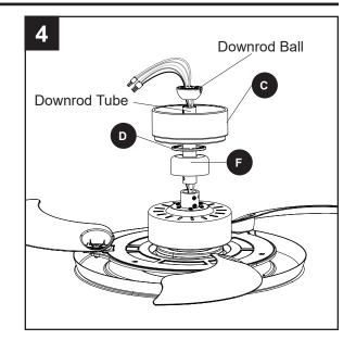
Loosen but do not remove the two set screws (I) in the yoke of the motor assembly (H). Slide the downrod tube into the yoke of the motor assembly (H), align the holes, then install the downrod pin and downrod clip from downrod pack (E). Retighten the two set screws (I) to secure the downrod. Then slide the yoke cover (F) down until it rests on top of the motor assembly (H).
