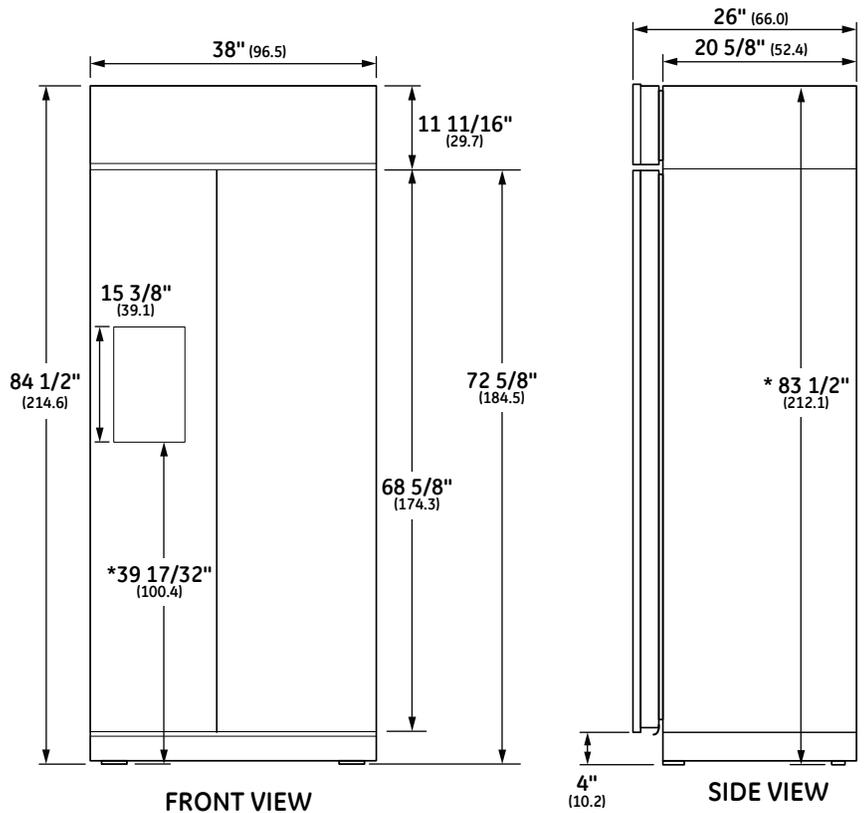
Use leveling legs and wheels for maximum 1" height adjustment from shipping height. Nominal installation height is 84".
