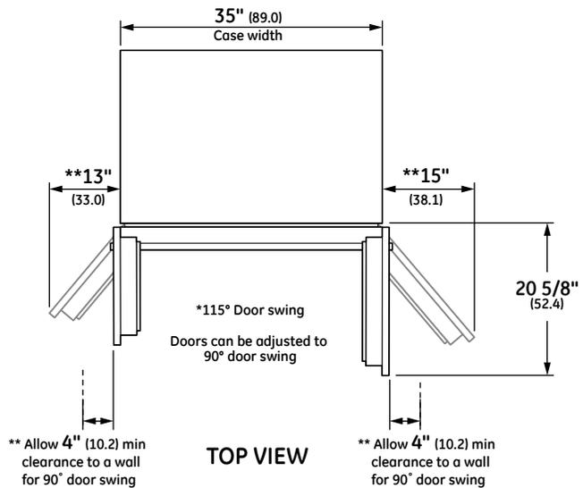
\*\* These refrigerators are equipped with a 2-position door stop. The factory-set 115° door swing can be adjusted to 90° if clearances to adjacent cabinets or walls is restricted. Allow a 15" minimum clearance to wall for pan removal. If the 90° door stop position is used, pan access is maintained, but pan removal is restricted.
