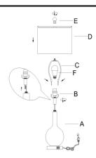
Step 1: Fasten Socket Assembly(B)onto Lamp body(A)
