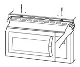
4. Remove the cover screw,pull the cover forward and then lift up the bulb holder.
