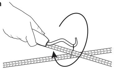
Fold the loop down to keep it from nearing the surface of the concrete.
