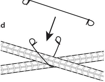
Insert the rebar tie tool into both loops and spin until the tie is tight.
