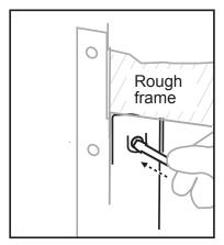
8. Pre-drill the hole in the upper tab with 9/64th-inch drill bit ensuring the drill bit goes on an upward angle through the vertical doorjamb, upper horizontal jamb and as far as possible into the upper rough frame. Secure the upper tab with the supplied 3-1/2 inch screw **G**.
