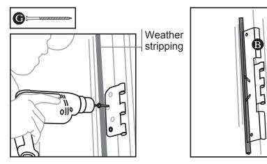
behind the weather stripping. When placed properly, the edge of the longer leg should be hidden by the weather stripping.
