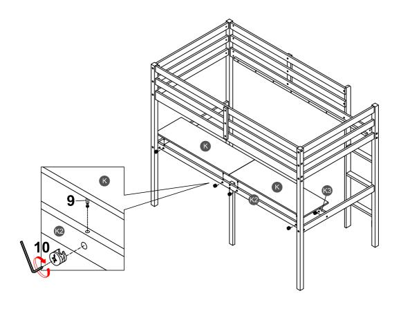
Note: Place hardware #10 with the "X" face outward, and make sure that the arrowhead is upward. Then, place hardware #10 into the hole of hardware #9 and tighten it clockwise with a hand screwdriver. (Please do NOT use an electric screwdriver.)
