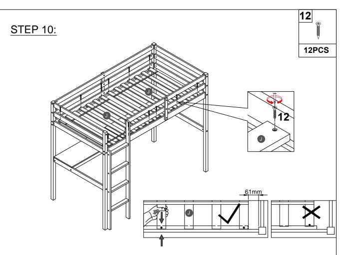
**NOTE:** Please make sure the bed slats close to the side rail before locking the screws to avoid breakage. This step is required for both the left and right sides. Moreover, please do not lock the screws of the bed slats at the outermost edge to avoid damaging.
