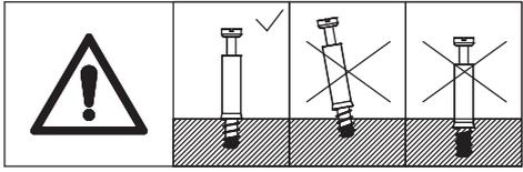
Fix board 10 to board 1 and 2 with screw(K) as shown.
