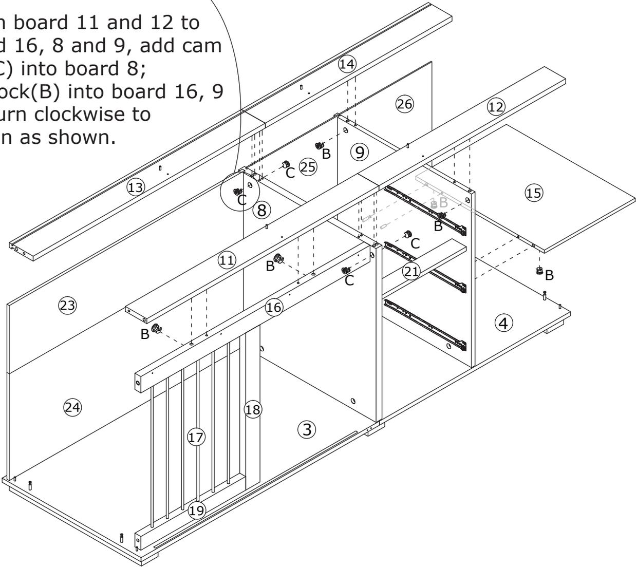
Attach board 15 to board 9, add cam lock(B) into board 15 and turn clockwise to tighten as shown.
