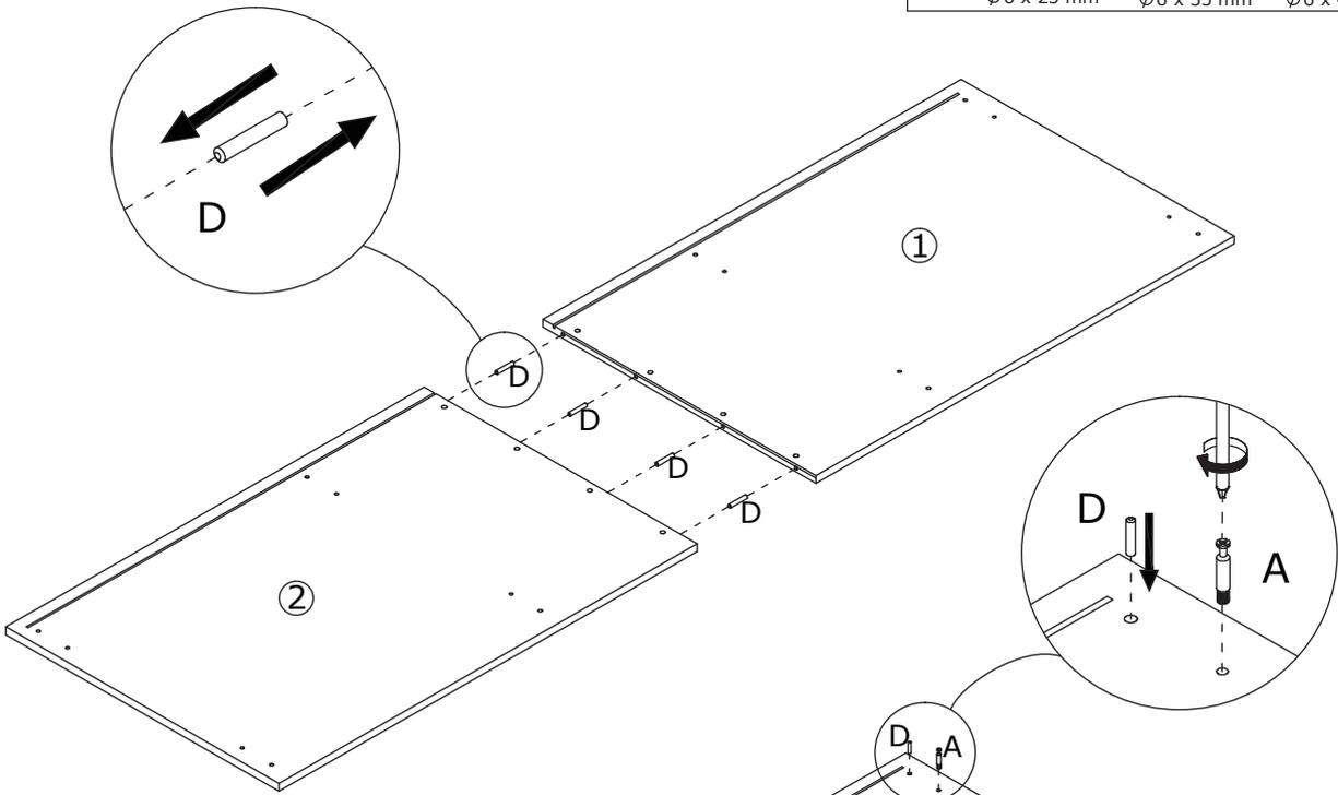
Screw eccentric rod(A) and insert wooden dowel(D) into board 2 and 1 at first.
