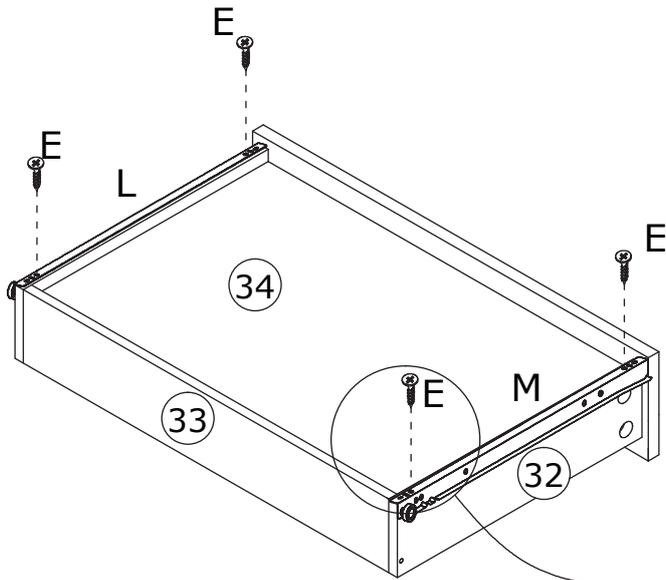
Fix runner(L) and (M) to board 31/36 and 32/37 with screw(E) as shown.
