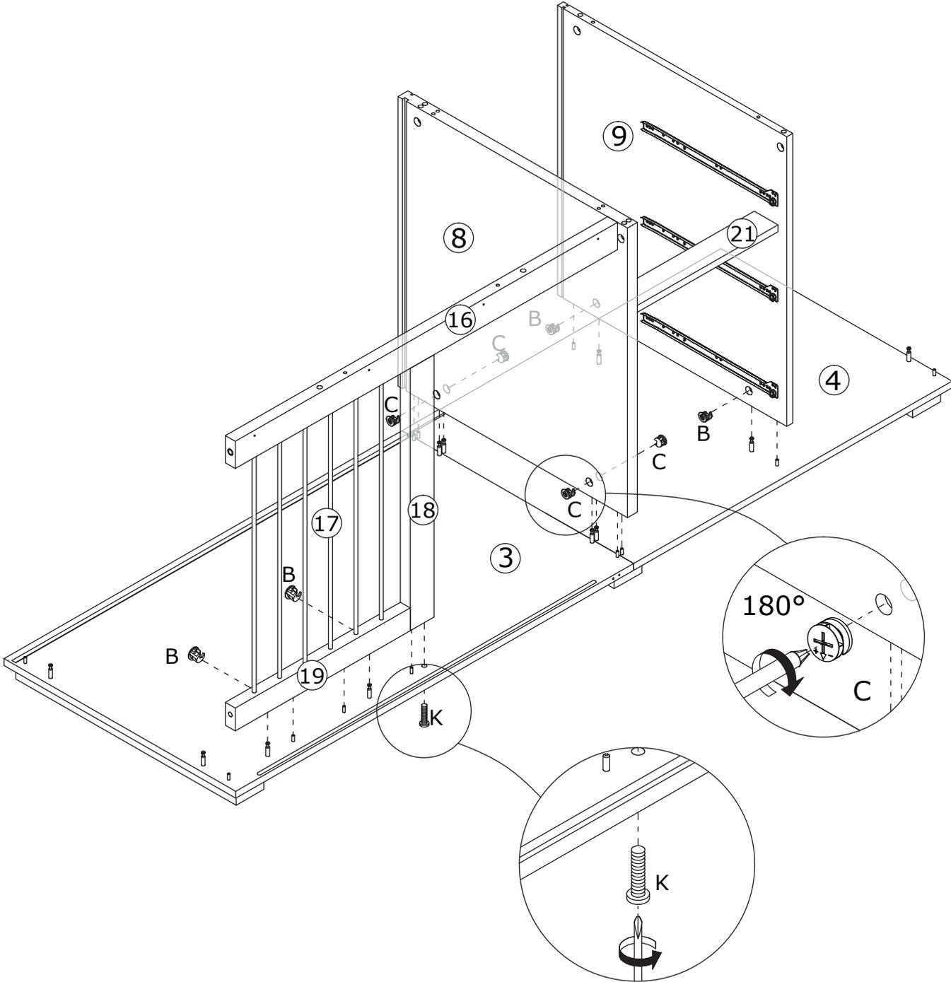
Fix board 18 to board 3 with screw(K) as shown.
