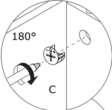
Attach board 13 and 14 to board 8 and 9, add cam lock(C) into board 8; cam lock(B) into board 9 and turn clockwise to tighten as shown.
