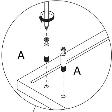
Screw eccentric rod(A) into board 30 and 35 as shown.
