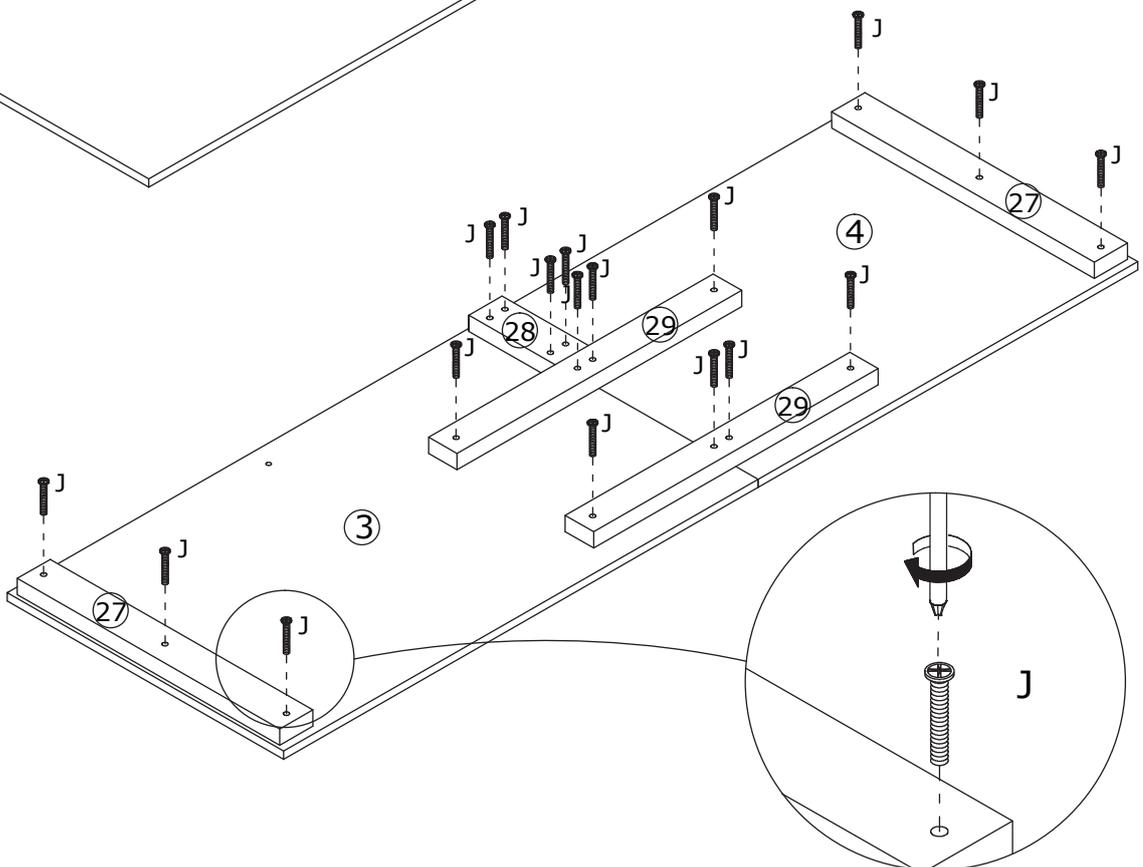
Fix board 27, 28 and 29 to board 3 and 4 with screw(J) as shown.
