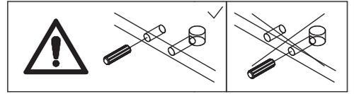
Connect board 23 to board 24 using wooden dowel(D) at first.
