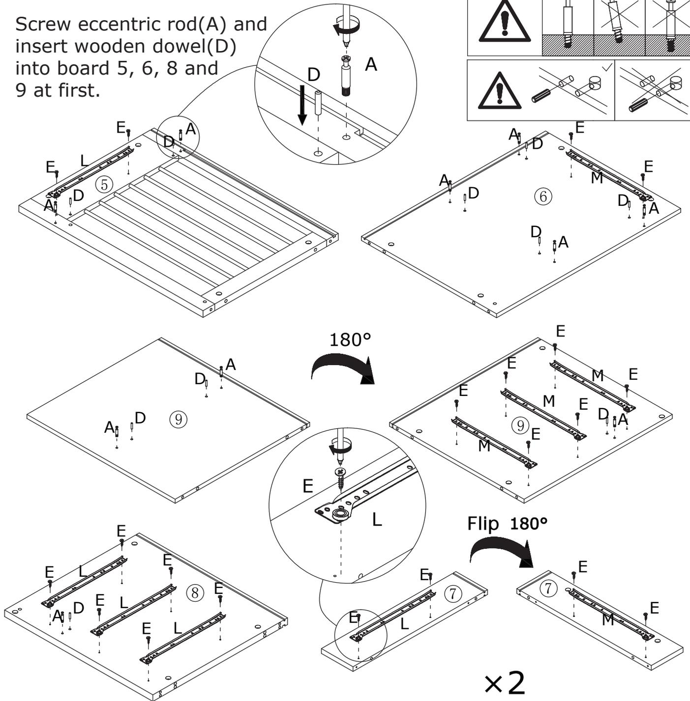
Fix slide rail(L) to board 5, 7 and 8 respectively with screw(E) as shown.
