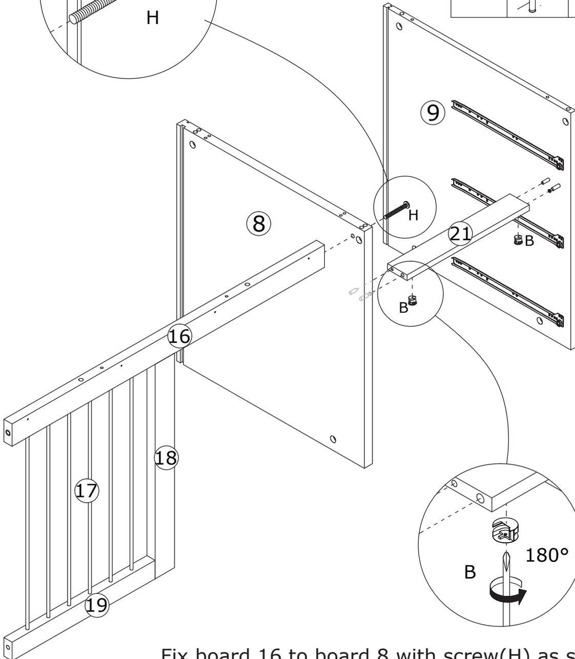
Fix board 16 to board 8 with screw(H) as shown.
