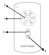
Fan **SPEED** buttons--1: Fan **OFF** button--2: **REVERSE** function button--3: **LIGHTING** button--4: Use to control ceiling fan speeds 1-6 Use to turn the fan off Use to control fan direction Use to control down-light and up-light (if applicable); Dims light when pressed and held down
