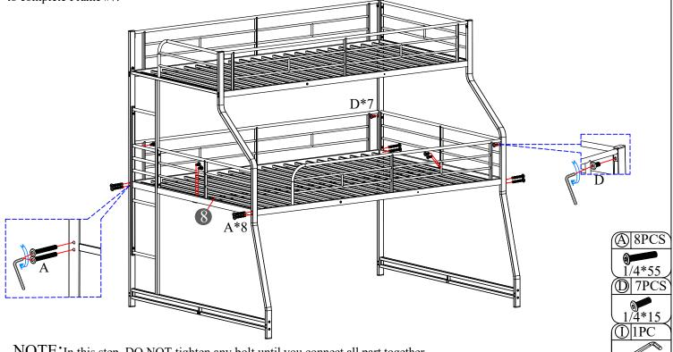
NOTE: In this step, DO NOT tighten any bolt until you connect all part together
