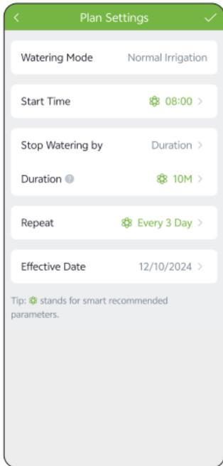
**Interval irrigation:** Set the run time for watering, interval time, start time, stop watering method, duration, frequency, and effective date. You can set the run time and interval time from 1s-60mins.
