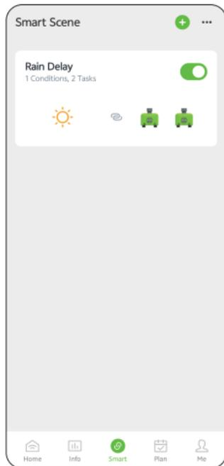
**For example:** The picture on the left shows that when the weather in New York is heavy rain, the left and right valves of the HTV245FRF WiFi irrigation timer will be automatically closed, and watering will be delayed for one day.
