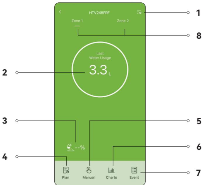
1. **Setting:** Tap the setting icon on the top right corner, you will enter the page for device setting, pair with soil sensor and customize the device watering.
