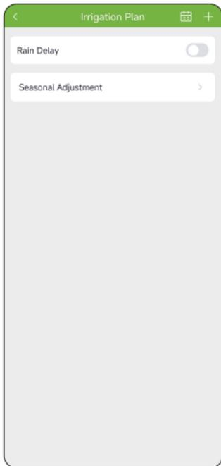
First tap the **"+"** icon on the top right corner of the **"Irrigation Plan"** page to choose your desired irrigation mode from **"Normal Irrigation"** **"Interval Irrigation"** **"Cycle & Soak"**.
