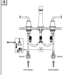
3.Connect the ④ inlet hose as shown, take note of the "Red" & "Blue" index from the handle. "Red" for connecting to the valve for supply hot water, and "Blue" for connecting to the valve for supply cold water.
