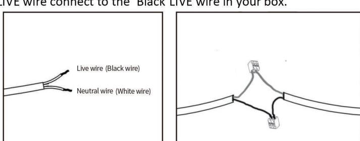
2, Connect the wire of the mirror to the wire of the plug and plug it into the socket
