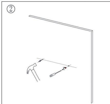
Insert the anchor and mounting screw
