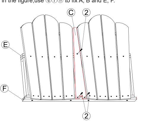
As shown in the figure, use 2 to fix C and E, F
