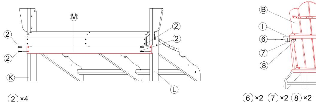
As shown in the figure,use ② to fix K, L and M
