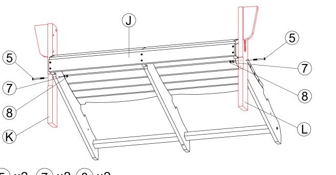
5) ×2 (7) ×2 (8) ×2 As shown in the figure,use 578 to fix K, L and J
