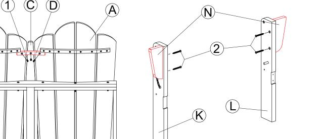
As shown in the figure, use ① to fix A, B, C and D
