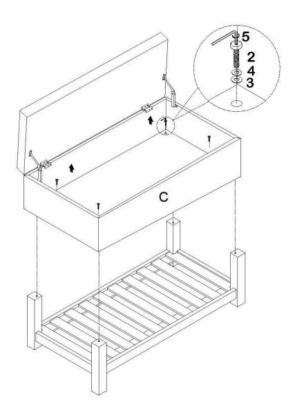
Place the Ottoman (A) on the assembled Shelf and Open the storage lid. Attach Ottoman (A) to Shelf with Allen Key Screws (2), Flat Washers (3) and Lock Washers (4).
