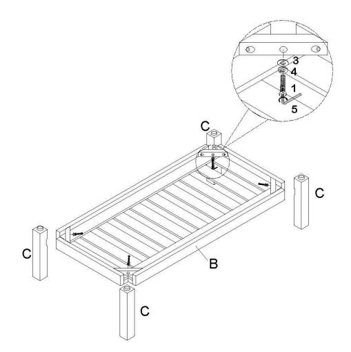
Assemble Legs (C) to the Shelf (B) with Allen Key Screws (1), Flat Washers (3) and Lock Washers (4). Use Allen Key (5) to tighten.
