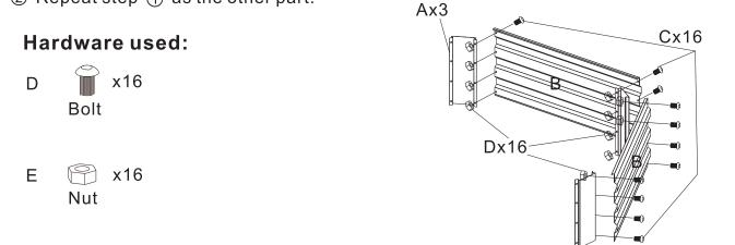
③ Attach two parts and panel (B) with bolts (C) and nuts (D).
