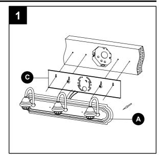
2. Using a 5/16 in. drill bit (not included), drill pilot holes at marked locations. For masonry installations, insert wall anchors (EE) into the holes. Otherwise, attach backplate (C) to wall using machine screws (DD) and use mounting screws (CC) to secure it to the outlet box.
