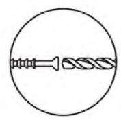
Match the drill bit to the wall anchor and hole size.
