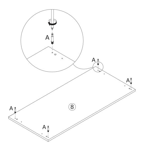
Insert quickfit screw A into panel 8 as shown. Please pay attention to the holes where the accessories are inserted and don't use an electric screwdriver.
