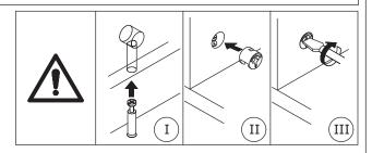
Connect 2 components, turn cam locks B clockwise to tighten as shown.
