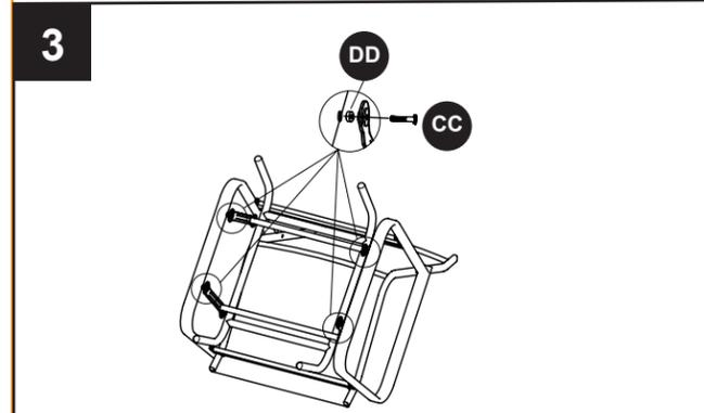
Once all connections are made, tighten CC, DD with EE.
