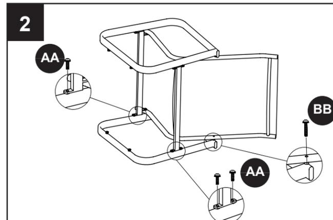
Once all connections are made, tighten AA, BB with EE.
