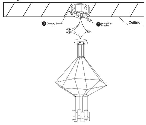
Attach canopy to mounting bracket (A). Twist canopy to lock fixture in place. Secure canopy with canopy screws (G).
