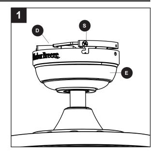
Secure the canopy (E) with the mounting bracket screws (S) previously removed (Step 4, page 8).
