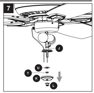
8. Lift the glass bowl (N) onto the threaded rod at the bottom of the light kit (J). Feed the pull chain coming from the grommet in the light kit (J) through the offcenter hole in the glass bowl (N). Feed pull chain coming from the center of the light kit (J) through the center hole in the glass bowl (N). Secure glass bowl (N) with rubber washer (U) and hex nut (T). Then attach finial cap (K) and finial (L).
