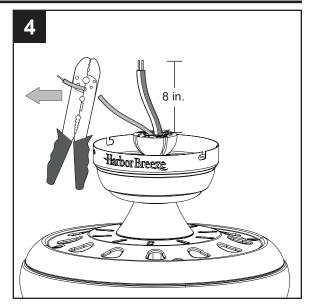
5. If you decided to cut back the lead wire in Step 4, strip 1/2 in. of insulation from the end of the white wire. Twist the stripped ends of each strand of wire within the insulation with pliers (not included). Repeat this step for black, blue and green wires.
