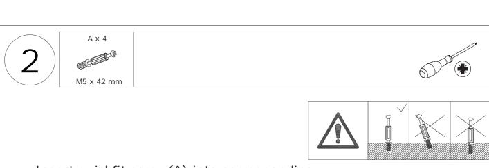
Insert quickfit screw(A) into corresponding holes in board 9 with a screwdriver as shown.
