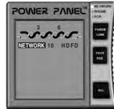
The NETWORK LED is lit. Press SEL to go to the NETWORK screen. The display says the device is transmitting on pair 3,6. The speed and duplex are indicated (10,100,1000,HD,FD). A "Force Link" button coerces a dialog.
