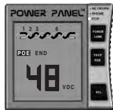
The POE LED is lit. Press SEL to go to the PoE screen. A PoE "end span" voltage of 48V is on pairs 1/2 & 3/6. If a lower "discovery" voltage is displayed, press "PoE Test" to simulate a PoE device and prompt the full 48VDC of PoE.
