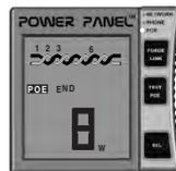
The POE LED is lit. Press SEL to go to the PoE screen. As in the above screen, the PoE voltage is on pairs 1/2 & 3/6. Watch the large digits. The first displayed is the PoE power draw in watts (8 watts shown). The second is the DC voltage amplitude (typically 48 VDC).
