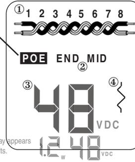
**NOTE ON POWER (WATT) DISPLAY:** To measure a device's power draw, the Power Panel must be connected inline (in between) the PSE switch and the PoE device.
