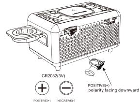
The lithium backup battery needs replacement when the LOW BATTERY indicator flashes, otherwise, the time and alarm settings will be lost/reset after a power outage
