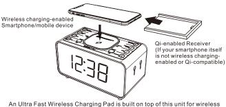
power transfer to any Qi-compatible smartphones or Qi-enabled receivers over a vertical distance of not more than 0.2 inches (5 mm). 1) Place your Qi-compatible smartphone or receiver (only one set at a
