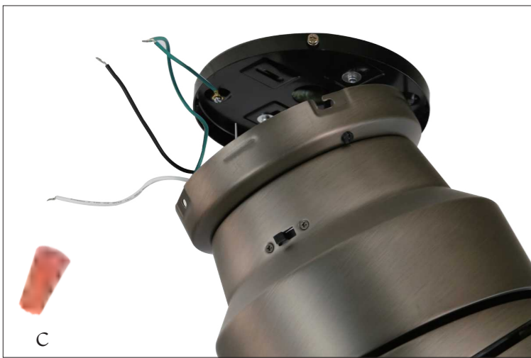
Step 4 Hang the motor to the J-hook on the mounting bracket. Connect the wires of the receiver to Home circuit. Black to Live wire, White to Neutral wire. Green to Ground wire.
