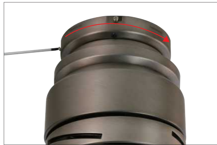
Step 5 Install the motor on the mounting plate. Rotate it until fixed. And then tighten 4 screws. Note: It is better to have a person to help you hold the motor when you install the screws to avoid dropping the motor.
