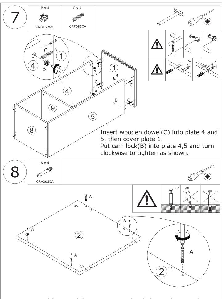
Insert quickfit screw(A) into corresponding holes in plate 2 with a screwdriver as shown.
