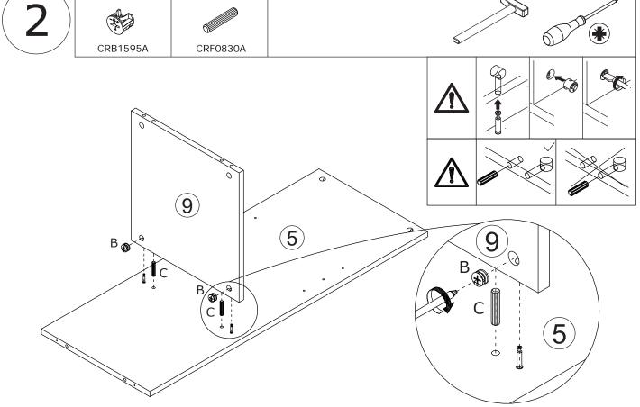
Insert wooden dowel(C) into plate 9, then attach to plate 5. Put cam lock(B) into plate 9 and turn clockwise to tighten as shown.  $^{5/14}$
