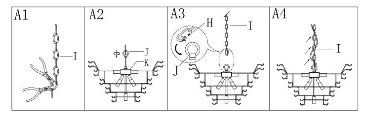
Step A1 » By measuring, determine the correct number of links needed for proper hanging height. Using the chain pliers, disconnect and discard the unwanted part.
