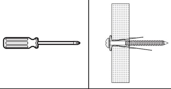
Screw wall anchors (H6) into the wall.
