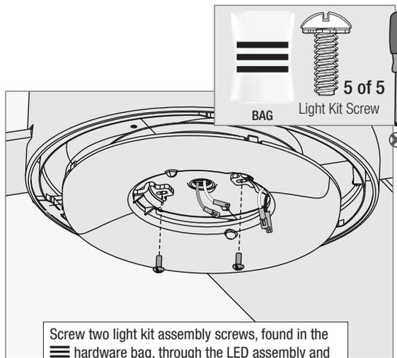
Screw two light kit assembly screws, found in the hardware bag, through the LED assembly and into the trim ring.
