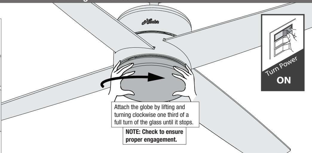
Attach the globe by lifting and turning clockwise one third of a full turn of the glass until it stops.
