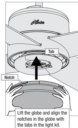
Lift the globe and align the notches in the globe with the tabs in the light kit.
