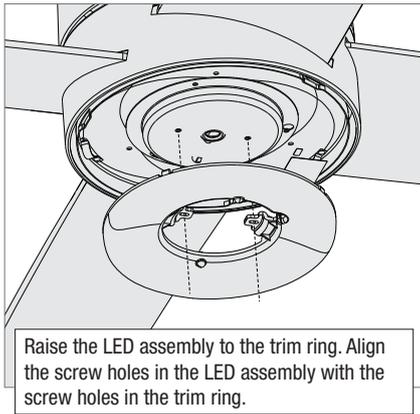
Raise the LED assembly to the trim ring. Align the screw holes in the LED assembly with the screw holes in the trim ring.
