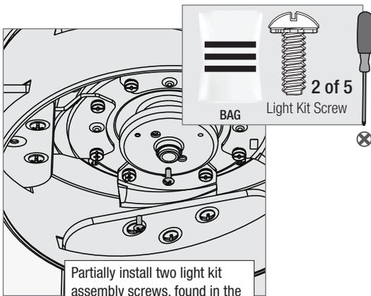
Partially install two light kit assembly screws, found in the hardware bag, halfway into the motor housing as shown. It does not matter which two screw holes you choose.
