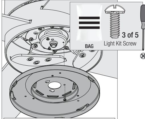
Align the keyhole slots in the top of the light kit assembly with the partially installed assembly screws. Wrap the keyhole slots around the screws and twist counterclockwise. Install the third screw. Tighten all three screws securely.
