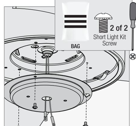
Feed the light wires through the hole in the lower switch housing. Align the lower switch housing screw holes with the bottom of the light kit assembly. Using the three Short Light Kit Screws, found in the hardware bag, mount the lower switch housing to the light kit.
