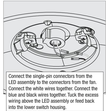
Connect the single-pin connectors from the LED assembly to the connectors from the fan. Connect the white wires together. Connect the blue and black wires together. Tuck the excess wiring above the LED assembly or feed back into the lower switch housing.
