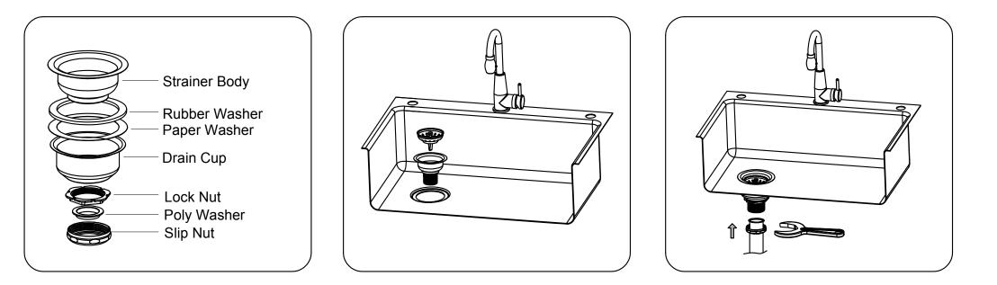
1. Remove the old sink strainer. Apply plumber's putty around the top of the sink drain hole. Position the strainer body in the sink opening and press down to secure it into position.
